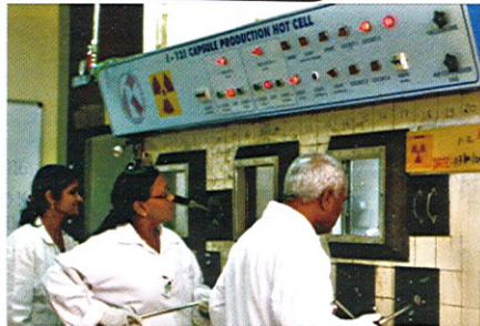
Iodine 131 capsule preparation in shielded hot cell
